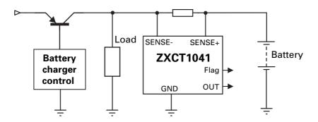
When choosing appropriate values for  $R_{\text{SENSE}}$  a compromise must be reached between in-line signal loss (including potential power dissipation effects) and small signal accuracy.
